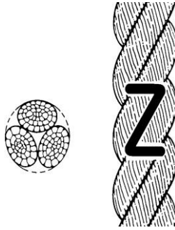
Figure 1 – Shape of a 3-strand hawser-laid rope (type A)
